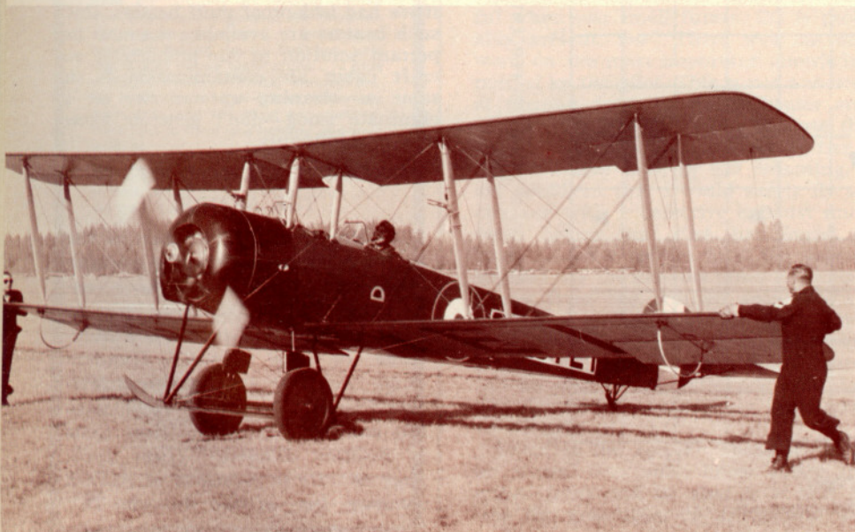
Wing-tip helpers walk a World War I "restored-pure" Avro 504K. It was necessary for helpers to maneuver this tail-skid, no-brakes antique safely across paved runway in a crosswind.
